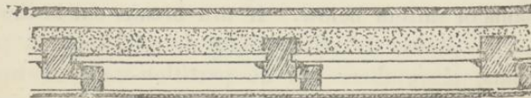
Fire-proof floor with filling and separate support for ceiling, and boarding between the beams.
